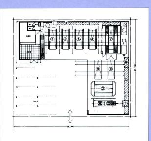
①②Body repair ③④Undercoating ⑤⑥Undercoating, Partial painting ⑦Top coating, Drying ⑧③Finish, Assembling (A) – (F) Place for materials & parts ⑥Compressor room
