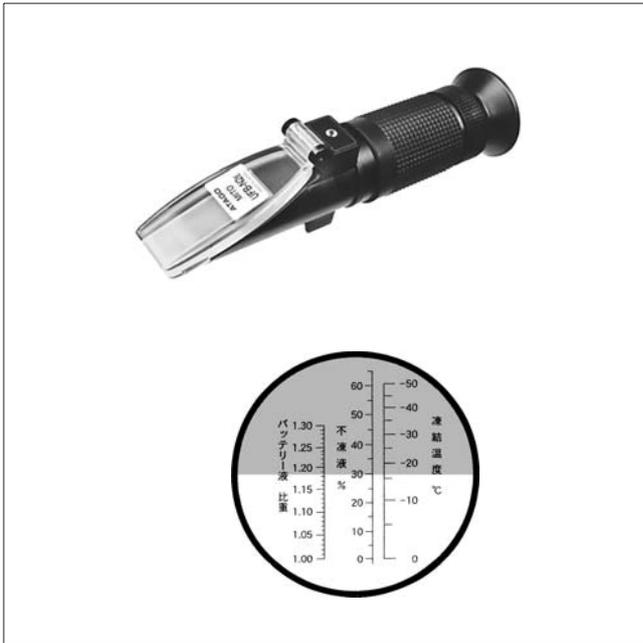
This is an optical hydrometer using a property of light such that the refractive index depends on the concentration of the liquid.
